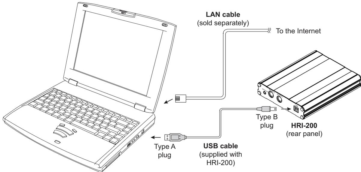
When the HRI-200 is connected to the PC properly, the HRI-200 will turn on automatically when the PC is turned on.
