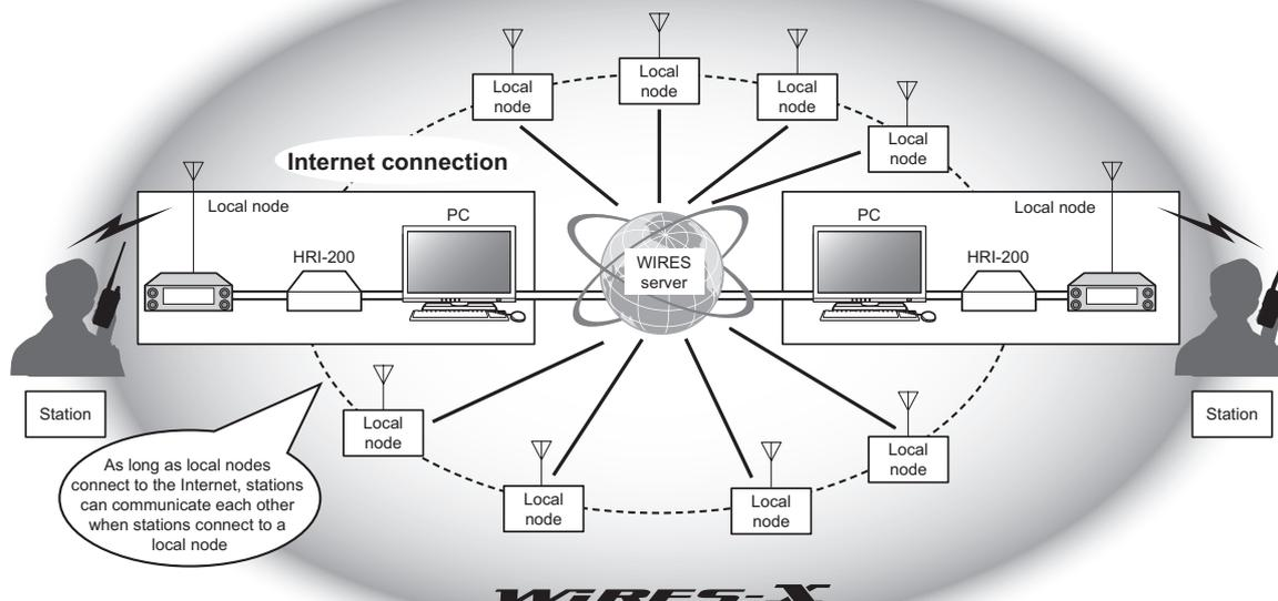
With the WIRES-X system, voice communication is carried out in the following manner:
