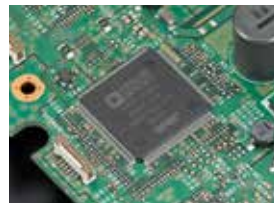
For band scope ADSP-21363 clock @333 MHz
