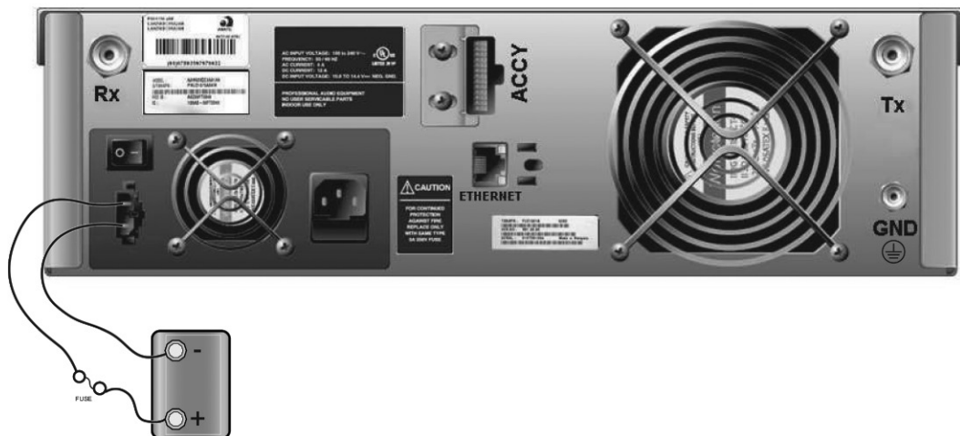
Figure 4-2: Making Connections to a Backup Battery
