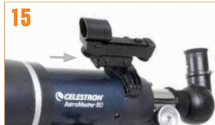
To install the finderscope on the 80AZS: Loosen the finger screw on the dovetail mount on the top left of the focuser. Slide the dovetail slider on the bottom of the finder bracket into the dovetail mount on the focuser. Tighten the finger screw to secure it in place.
