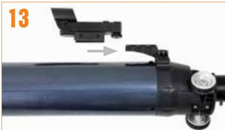
To install the finderscope on the 70AZ, 90AZ, and 102AZ: Loosen the two Philips-head screws on the side of the finderscope and slide the clamp over the dovetail bracket. Secure the finderscope in place by tightening the two Philips-head screws.
