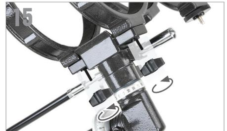
Align the holes on the bottom half tube rings with the holes on the mount and secure them in place with the black wing nuts removed in step 14.
