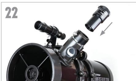
For additional magnification, you can use the included 3x Barlow Lens. Place the Barlow lens in the focuser in place of the eyepiece. Remove the cap from the Barlow lens.
