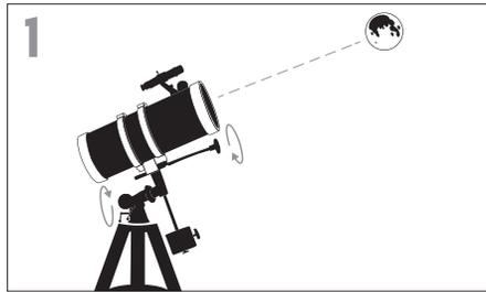
With the Moon visible in the sky, set up your telescope as described above with the 20mm eyepiece installed. Move the telescope so that it is roughly pointing toward the Moon.
