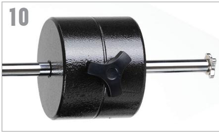
Locate the counterweight bar and counterweight. Slide the counterweight half way down the counterweight bar.
