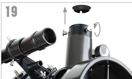
Loosen the set screws on the focuser so they do not obstruct the inner diameter of the focuser. Remove the plastic cap covering the end of the focuser.
