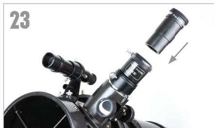
Next, insert the eyepiece into the Barlow and tighten the set screws to secure it in place.
