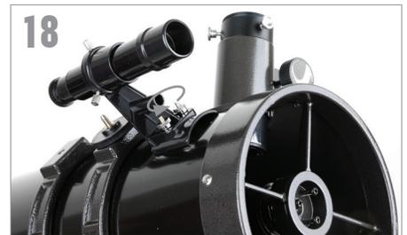
Locate the finderscope and remove plastic caps on front and back of lens. Orient the finderscope so that the glass window is facing towards the front of the tube as shown here. Place finderscope over the posts on the tube and tighten it down with the knurled nuts.
