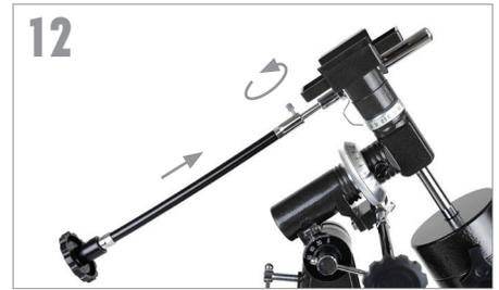
Slide the chrome end of the slow motion control cables onto equatorial mount gear shaft. Be sure to line up the set screw over the flat spot on the shaft. Tighten screw to secure in place.
