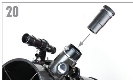
Insert the barrel of the 20mm eyepiece into the focuser and tighten the screws.
