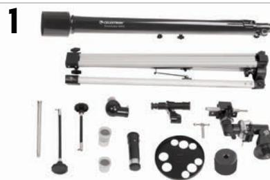
Unpack your telescope and verify that all parts are present. Your PowerSeeker 60EQ includes: an optical tube, a tripod, an equatorial mount, a latitude adjustment screw, a diagonal, two eyepieces, a 3x Barlow lens, a finderscope, a 2 lb. counterweight, a counterweight bar, two slow motion cables, and an eyepiece accessory tray.
