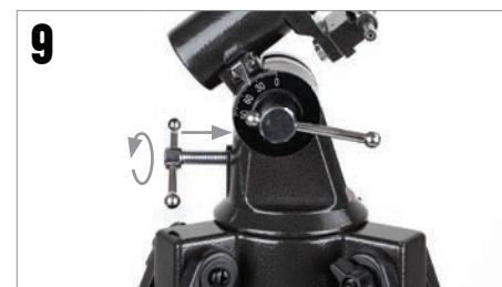
Look up the approximate latitude of your observing site on the Internet or using a map. Then, thread the latitude adjustment screw into the equatorial mount until your latitude is indicated on the latitude scale.
