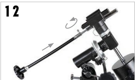
Slide the chrome end of the slow motion control cables onto equatorial mount gear shaft. Be sure to line up the set screw over the flat spot on the shaft. Tighten screw to secure in place.
