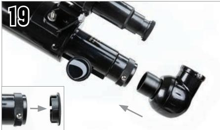
Loosen the screws on the focuser so they do not obstruct the inner diameter of the focuser. Insert diagonal into the focuser and tighten the set screws. Remove the plastic cap covering the end of the focuser.
