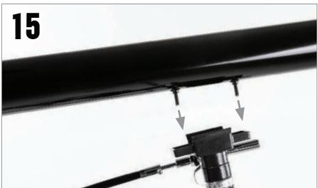
Place the tube on the mount by lining up the screws with the mounting holes on the mount.
