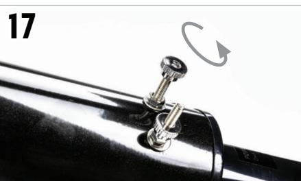
Remove the knurled nuts at the focuser end of the telescope tube.
