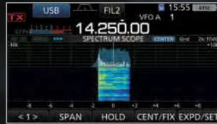
DPD ON (Signal Received on the IC-7300) No spurious emission observed
