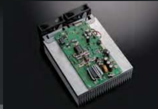
PA Unit with a Large Heatsink
