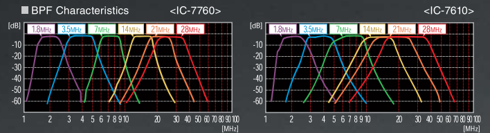
Showing primary BPF for HF amateur bands
