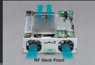
Effective Cooling System with Four Fans
