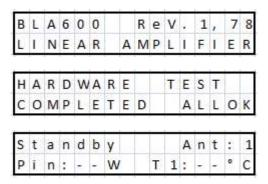
After this has taken place the amplifier will be 'Standby' mode. A test transmission can now be made to ensure that there is no problem with any of the connections. During this time the amplifier will read the transmit frequency and automatically change to the correct Low Pass Filter, which will be indicated on the front panel by illuminating the relevant band indicator  $\Phi$ . (The correct band filter may also be
