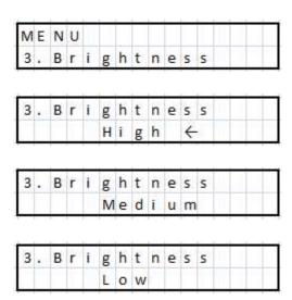
Change the intensity of the LCD backlight, LED Power Meter, LED SWR Indicator. There are 3 options, Low, Medium and High. Select menu '3:Brightness' with the 'Navigate' key then press 'Enter' key to access the menu. You can now use the '+' key to increase the brightness or the '-' key to decrease the brightness. Press 'Enter' to save the current selection and return to the menu list.
