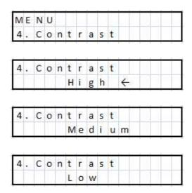
Change the contrast of the LCD display. There are 3 options Low, Medium and High. Select menu '4:Contrast' with the 'Navigate' key ? Press 'Enter' key ? to access the menu. You can now use the '+' key ? to increase the contrast and the '-' key to reduce the contrast. After selection, press the 'Enter' key ? to save the current selection and return to the menu list.
