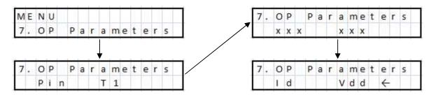
Use the 'Navigate' key **7** to select menu '7:TX Parameters'. Press the 'Enter' key to access the menu and use the '+' **6** and '-' **6** keys to choose from the above ten choices. Press the 'Enter' key **4** again to save the current selection and return to the menu list.
