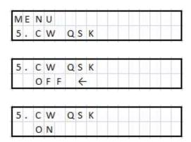
To minimise the RTX switching time for maximum performance in 'Full Break In' mode, especially if sending 25+WPM this menu should be activated. Use the 'Navigate' key to select '5:CW QSK' and then press the 'Enter' key to access the menu. Use '+' or '-' keys to select 'On' or 'Off'. Then press the 'Enter' key to save the current selection and return to the menu list. When returning to 'Operate' mode the LCD display will have changed to:
