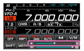
Turn the **mouse wheel**, or drag or click on the slide bar to adjust the receive audio to a comfortable volume.
