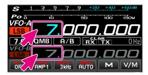
Wheel: Move frequency Up / down at 1MHz
