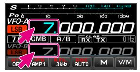
2. In this state, turning the mouse wheel will change the frequency in 1MHz steps.
