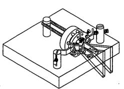
Vary contact spacing to suit your personal preference by loosening the set screws in the split posts (with wrench provided) and turn the contact screw to the desired spacing. Re-tighten the set screw.
